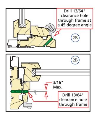
PLACEMENT DIAGRAM (For placement of Frame Screws and Installation Clips)
